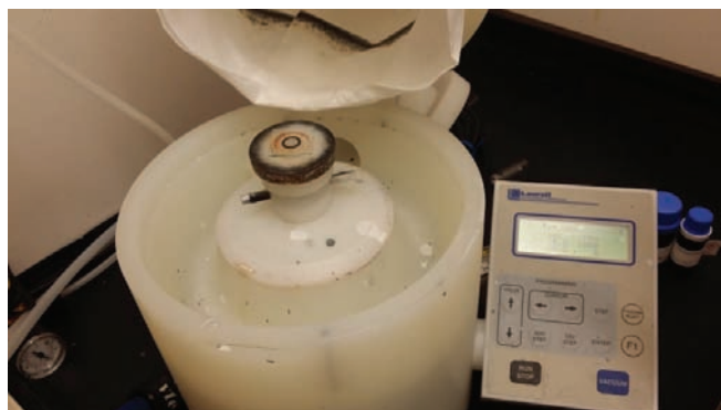
Figure 4: Spin coating machine in which metal oxide NPs were applied at various revolutions per minute when making HTLs.
